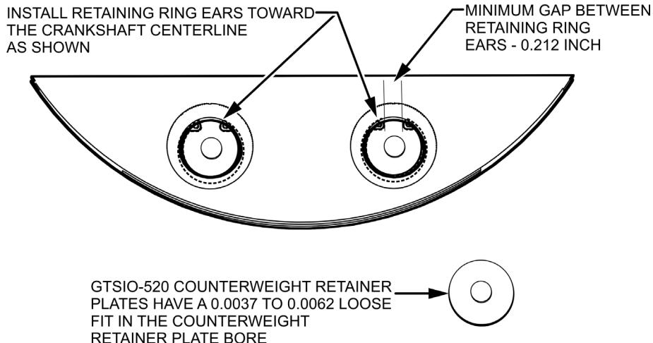
**Figure 3. Counterweight Inspection**
