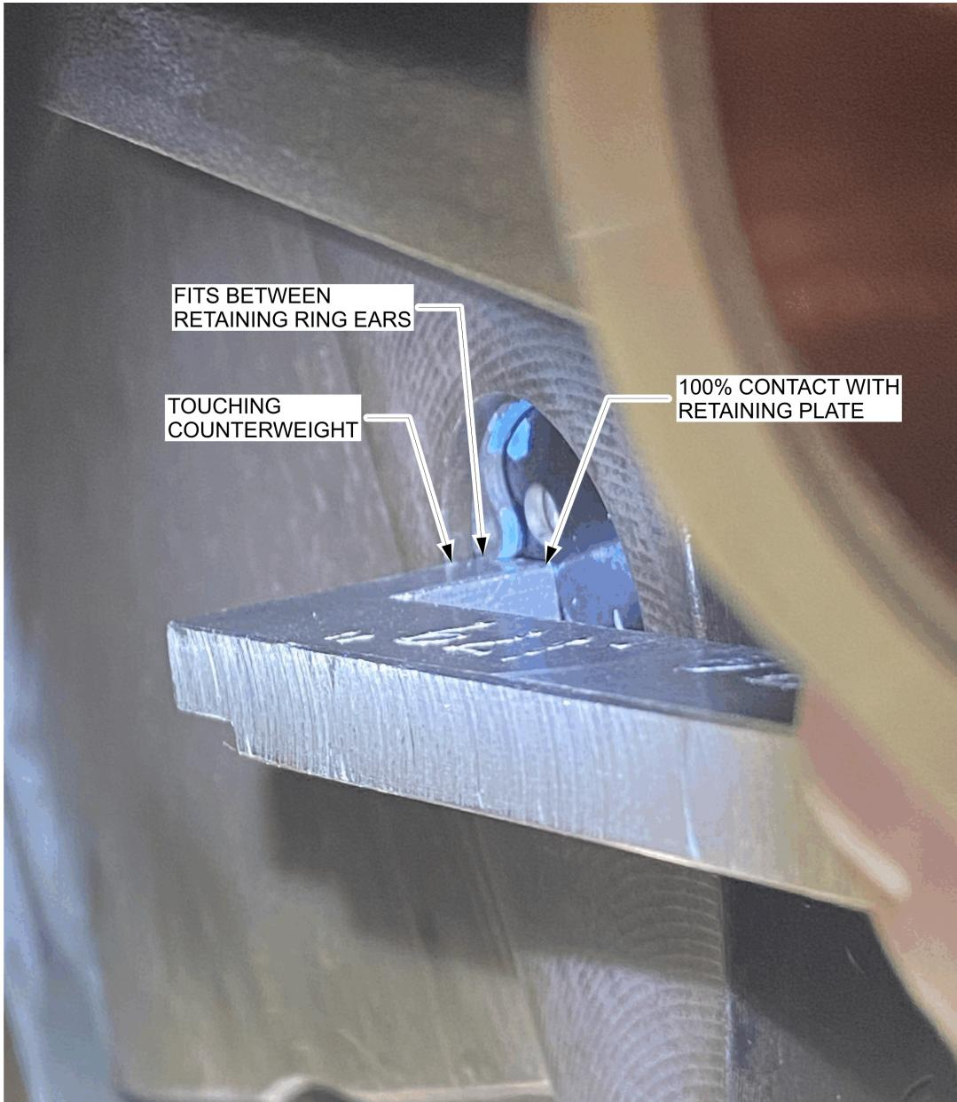
Figure 1. Gage Inserted to Measure Retaining Ring Gap
