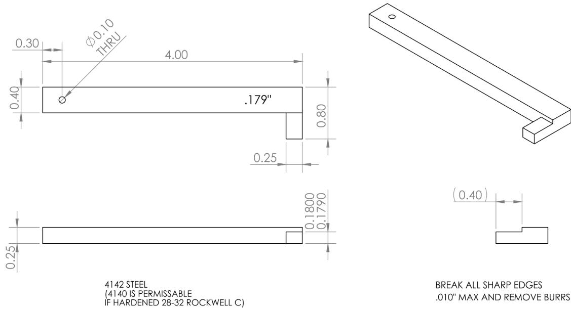
Figure 4. 0.179 Inch Gage (470, IO520, L/TSIO-520, and 550 Series Engines Only)
