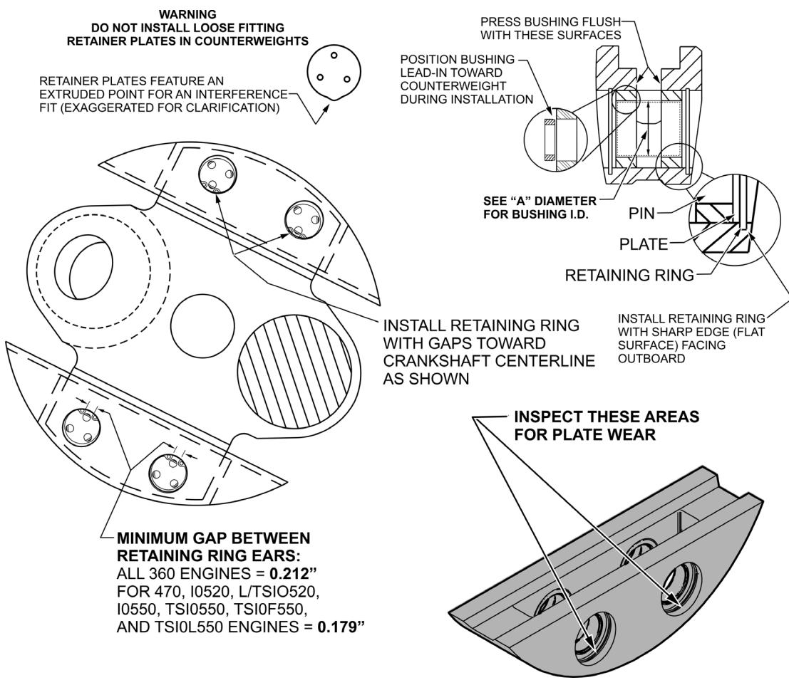
**Figure 2. Counterweight Inspection**
