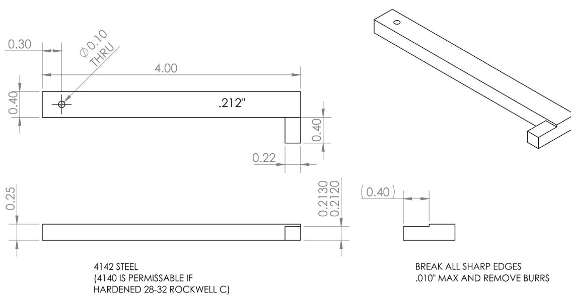
Figure 5. 0.212 Inch Gage (IO/LTSIO/TSIO-360 and GTSIO-520 Series Engines Only)
