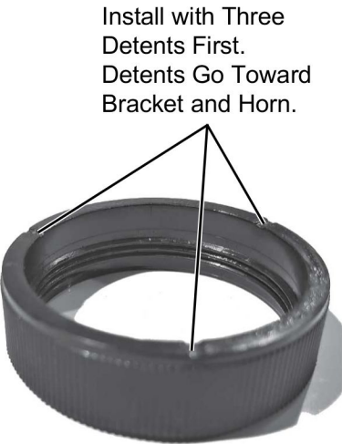
DETAIL C Knurled Nut Install Direction
