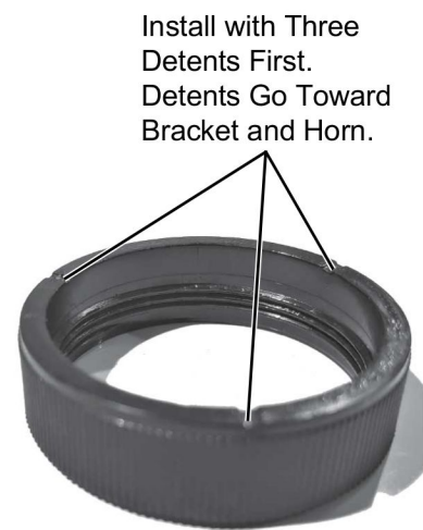
DETAIL C Knurled Nut Install Direction
