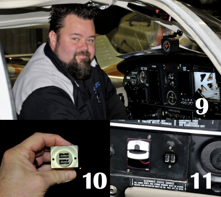
Above from top: A&P/IA Erich Rempert about to configure the engine monitor. • Guardian Avionics dual USB power port. • Guardian Avionics pulse oximeter monitor (left) and USB power port installed in Scott's panel.
