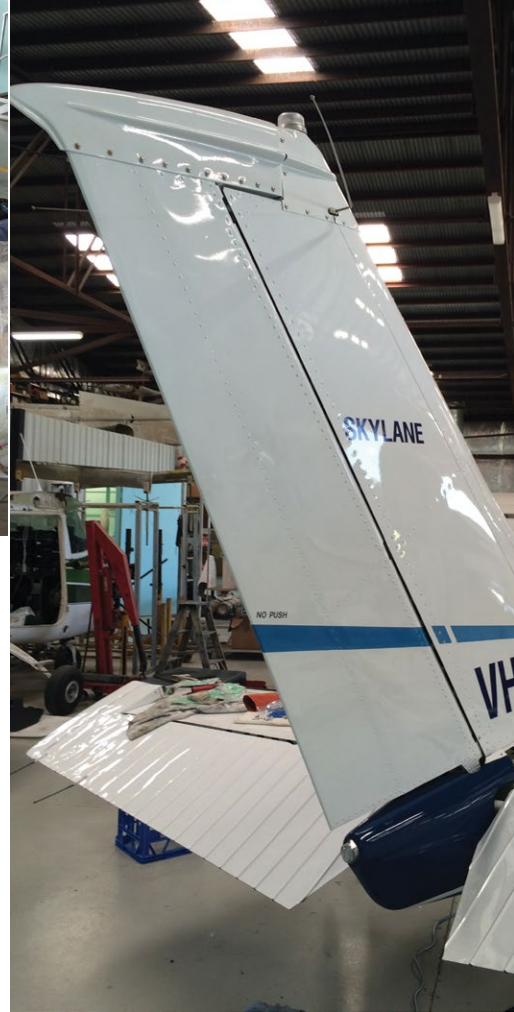
Since the tail section of the Skylane was out in the elements, it suffered the worst corrosion and had to be partially rebuilt.
