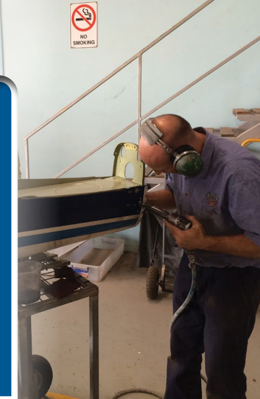
The airframe suffered extensive corrosion and several sections had to be replaced including a few ribs in the tail section and the aft carry-through spar.
