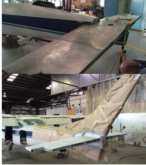
Since the tail section of the Skylane was out in the elements, it suffered the worst corrosion and had to be partially rebuilt.
