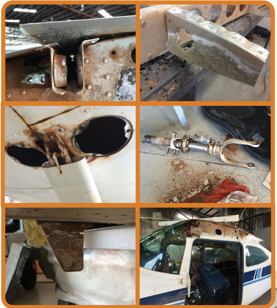
The airframe suffered extensive corrosion and several sections had to be replaced including a few ribs in the tail section and the aft carry-through spar.
