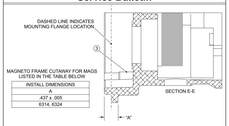
USE A CALIBRATED MEASURING DEVICE TO MEASURE DISTANCE "A", AS SHOWN IN CUTAWAY SECTION E-E. MAKE SURE THE FRAME SURFACE IS FREE OF CONTAMINANTS. ANY MEASUREMENT LESS THAN 0.432 INCH OF ANY PART OF THE STOP PIN (3), THE MAGNETO SHOULD BE REMOVED FROM SERVICE AND RETURNED TO CHAMPION FOR WARRANTY.
