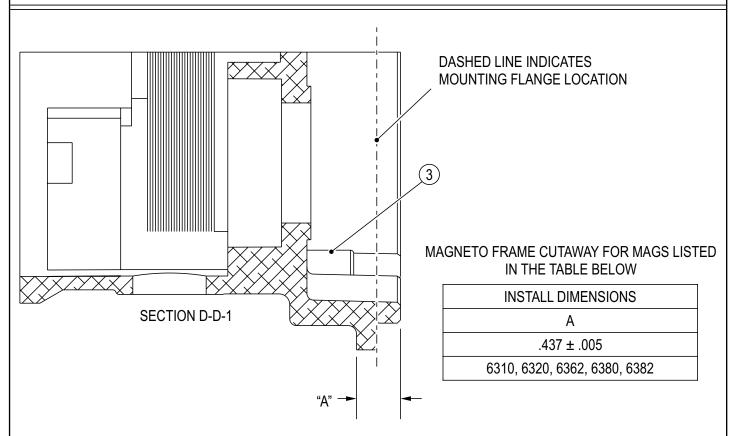
USE A CALIBRATED MEASURING DEVICE TO MEASURE DISTANCE "A", AS SHOWN IN CUTAWAY SECTION D-D-1. MAKE SURE THE FRAME SURFACE IS FREE OF CONTAMINANTS. ANY MEASUREMENT LESS THAN 0.432 INCH OF ANY PART OF THE STOP PIN (3), THE MAGNETO SHOULD BE REMOVED FROM SERVICE AND RETURNED TO CHAMPION FOR WARRANTY.
