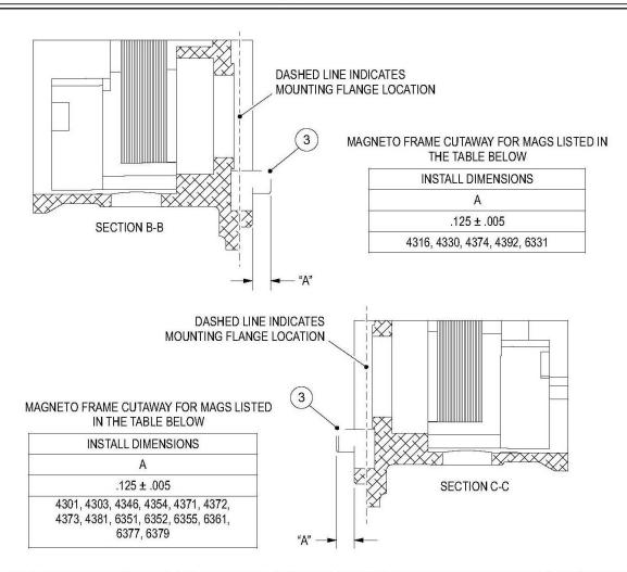
USE A CALIBRATED MEASURING DEVICE TO MEASURE DISTANCE "A", AS SHOWN IN CUTAWAY SECTIONS B-B AND C-C. MAKE SURE THE FRAME SURFACE IS FREE OF CONTAMINANTS. ANY MEASUREMENT GREATER THAN 0.130 INCH OF ANY PART OF THE STOP PIN (3), THE MAGNETO SHOULD BE REMOVED FROM SERVICE AND RETURNED TO CHAMPION FOR WARRANTY.
