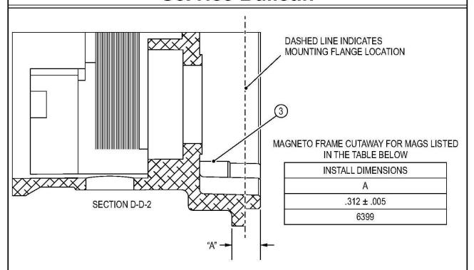
USE A CALIBRATED MEASURING DEVICE TO MEASURE DISTANCE "A", AS SHOWN IN CUTAWAY SECTION D-D-2. MAKE SURE THE FRAME SURFACE IS FREE OF CONTAMINANTS. ANY MEASUREMENT LESS THAN 0.307 INCH OF ANY PART OF THE STOP PIN (3), THE MAGNETO SHOULD BE REMOVED FROM SERVICE AND RETURNED TO CHAMPION FOR WARRANTY.
