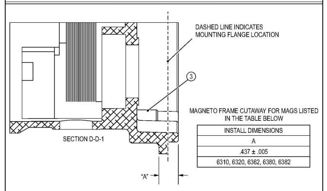
USE A CALIBRATED MEASURING DEVICE TO MEASURE DISTANCE "A", AS SHOWN IN CUTAWAY SECTION D-D-1. MAKE SURE THE FRAME SURFACE IS FREE OF CONTAMINANTS. ANY MEASUREMENT LESS THAN 0.432 INCH OF ANY PART OF THE STOP PIN (3), THE MAGNETO SHOULD BE REMOVED FROM SERVICE AND RETURNED TO CHAMPION FOR WARRANTY.
