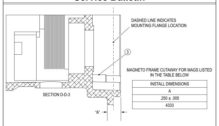
USE A CALIBRATED MEASURING DEVICE TO MEASURE DISTANCE "A", AS SHOWN IN CUTAWAY SECTION D-D-3. MAKE SURE THE FRAME SURFACE IS FREE OF CONTAMINANTS. ANY MEASUREMENT LESS THAN 0.245 INCH OF ANY PART OF THE STOP PIN (3), THE MAGNETO SHOULD BE REMOVED FROM SERVICE AND RETURNED TO CHAMPION FOR WARRANTY.
