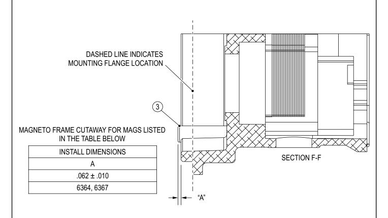
USE A CALIBRATED MEASURING DEVICE TO MEASURE DISTANCE "A", AS SHOWN IN CUTAWAY SECTION F-F. MAKE SURE THE FRAME SURFACE IS FREE OF CONTAMINANTS. ANY MEASUREMENT GREATER THAN .072 INCH OF ANY PART OF THE STOP PIN (3), THE MAGNETO SHOULD BE REMOVED FROM SERVICE AND RETURNED TO CHAMPION FOR WARRANTY.
