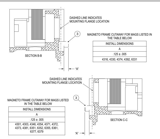
USE A CALIBRATED MEASURING DEVICE TO MEASURE DISTANCE "A", AS SHOWN IN CUTAWAY SECTIONS B-B AND C-C. MAKE SURE THE FRAME SURFACE IS FREE OF CONTAMINANTS. ANY MEASUREMENT GREATER THAN 0.130 INCH OF ANY PART OF THE STOP PIN (3), THE MAGNETO SHOULD BE REMOVED FROM SERVICE AND RETURNED TO CHAMPION FOR WARRANTY.
