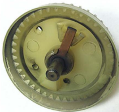
Figure 3. Affected K3008 Distributor Gear With Copper Electrode
