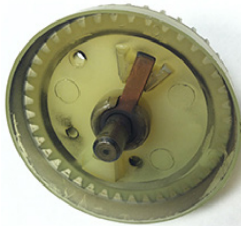
Figure 3. Affected K3008 Distributor Gear With Copper Electrode
