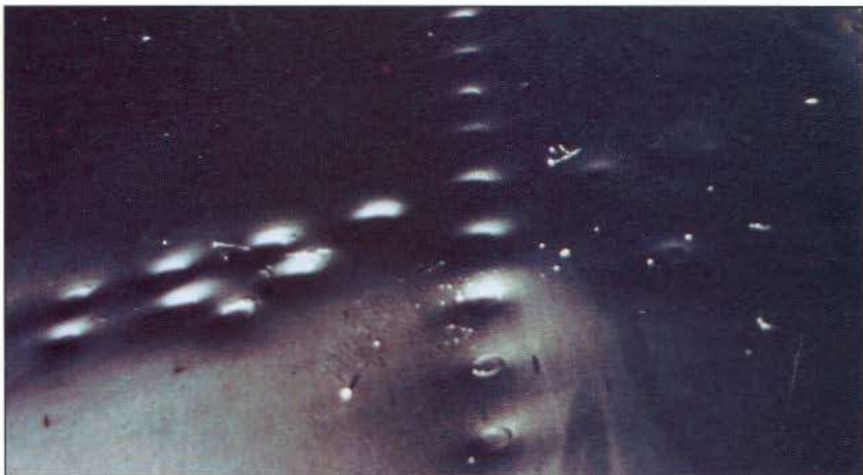
FIGURE 4-12. SKIN BULGING AROUND FASTENERS
