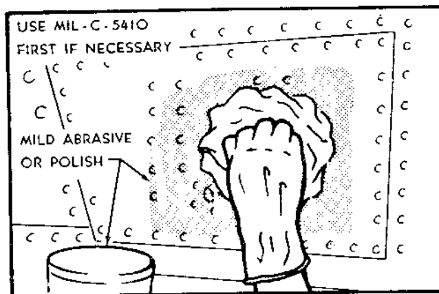
FIGURE 6-12. POLISHING AND BRIGHTENING ALCAD SURFACES
