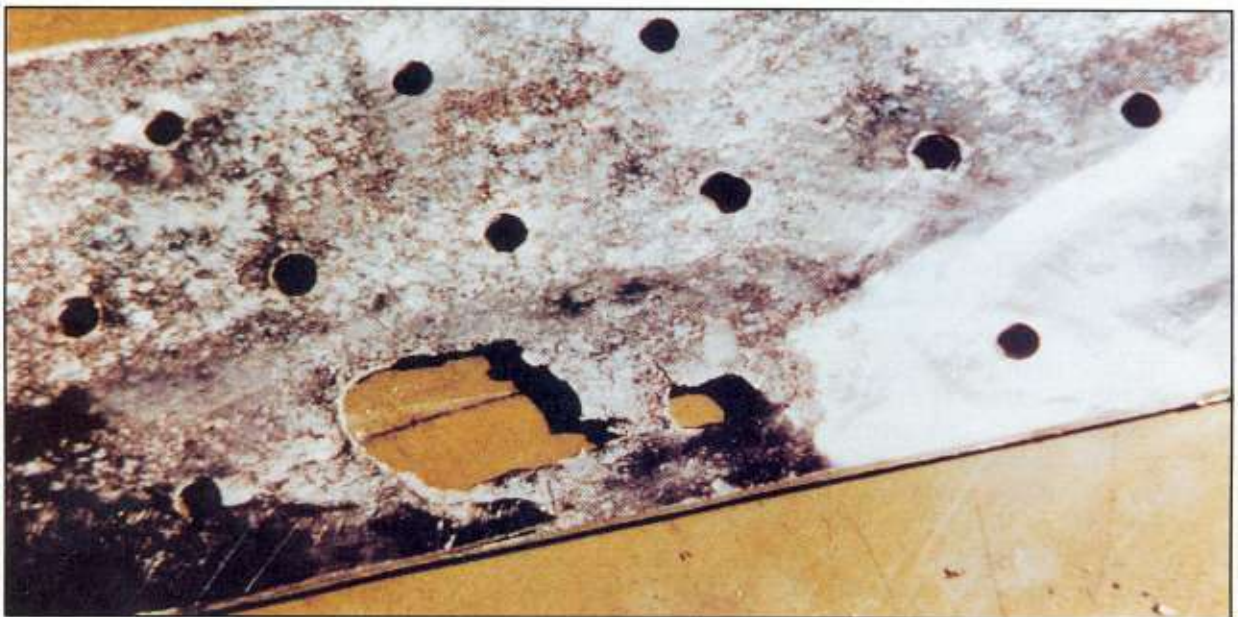
FIGURE 6-8. SEVERE CORROSION REQUIRING TRIMMING OUT OF DAMAGED AREA
