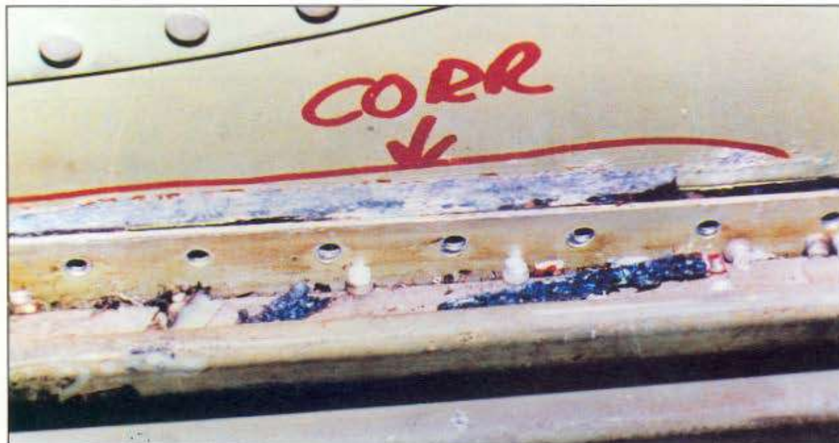
FIGURE 5-10. REMOVAL OF FILLET SEAL FROM INTERNAL EDGE OF LAP JOINT EXPOSED FULL EXTENT OF CORROSION
