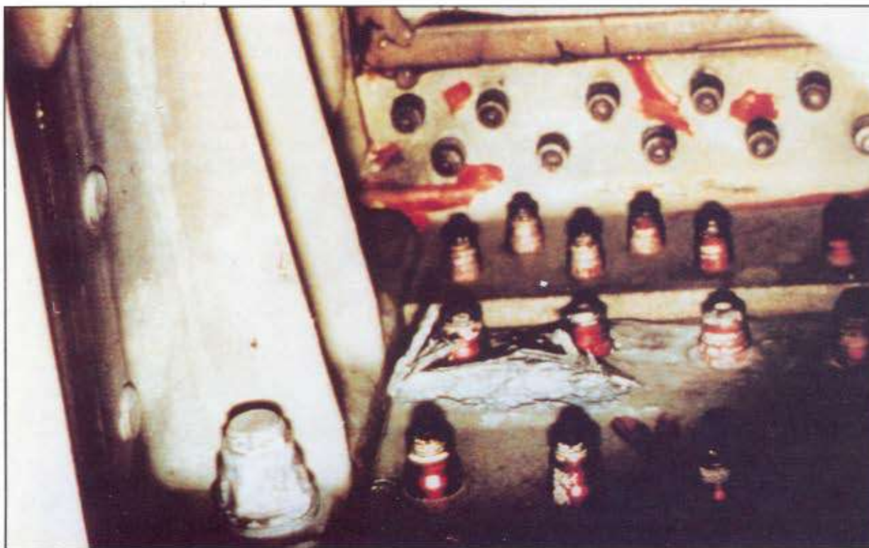
FIGURE 2-9. SEVERE EXFOLIATION CORROSION
