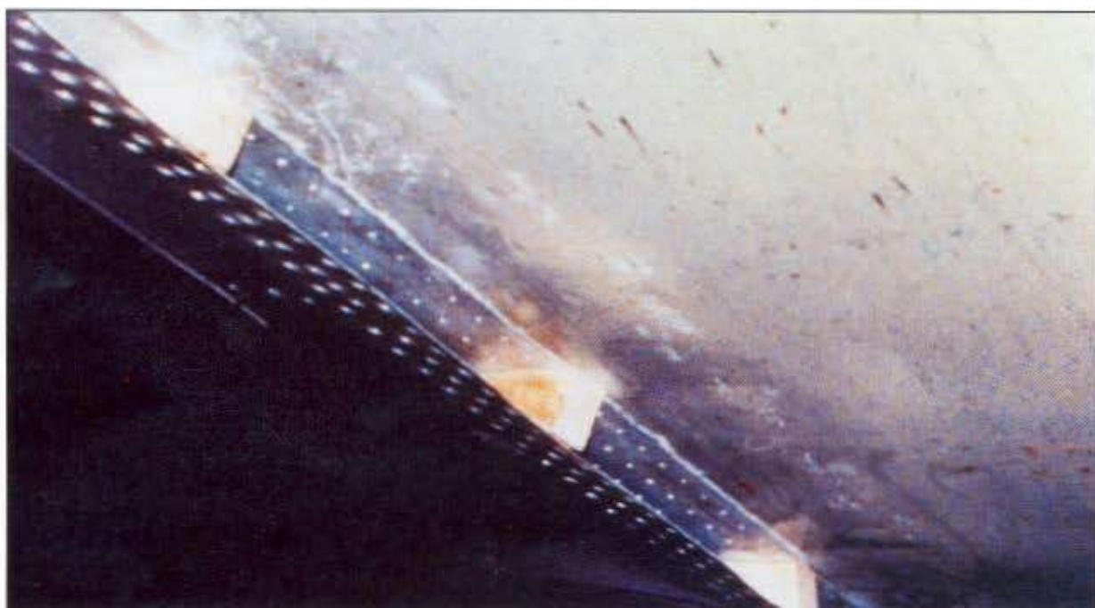
FIGURE 4-13. OPENING OF A CORRODED LAP JOINT FOR REPAIR
