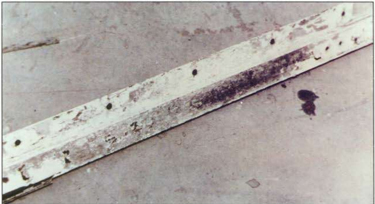
FIGURE 2-3. UNIFORM ETCH CORROSION
