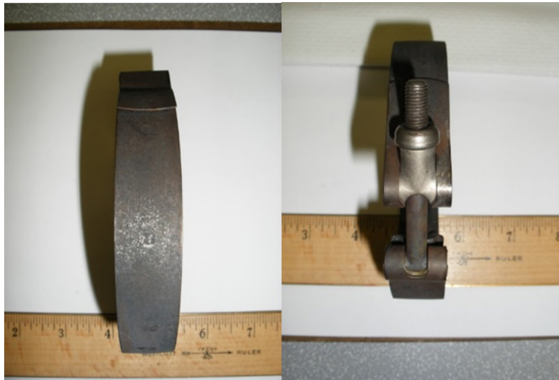
Figure 24 Spot-welded, 3-segment, Coupling
