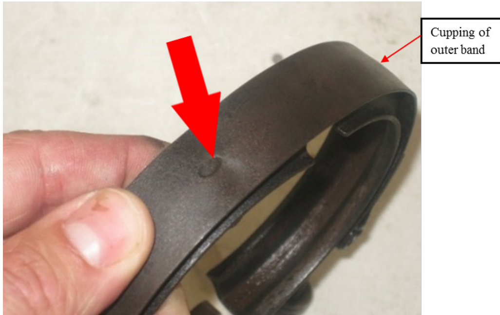
Figure 22 Spot-welded, 3-segment Coupling
